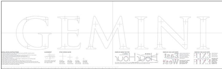
**DRILL PATTERN:** (for all other stud mounted products) Computer-generated tracing of letters with hand punched hole locations of studs, printed on 60# white grid paper. Once taped to wall, hole locations are then drilled and filled with adhesive.
