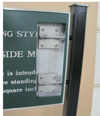
Double face side mount plaques have ss plates and projecting ss studs bolted into the plaque during manufacturing. The projecting ss studs will be used to bolt the posts to the plaque. Assembling is done by laying the plaque with one face down on a suitable surface
